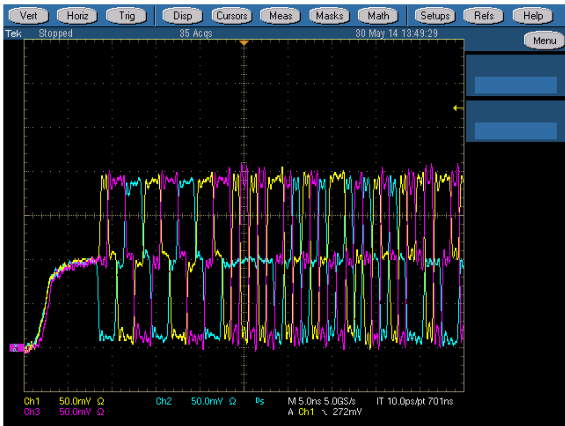
ATx 1.3 Transmitter: Packet through header Yellow: Wire A; Blue: Wire B; Magenta: Wire C Corresponding Received waveform below Yellow: A-B; Blue: B-C; Magenta: C-A
