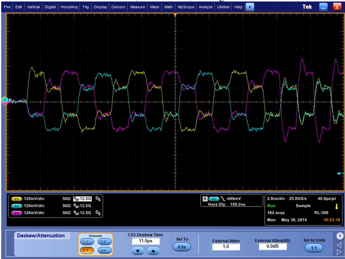
ATx 1.1 Transmitter beginning of HS data – preamble Yellow: Wire A; Blue: Wire B; Magenta: Wire C Corresponding Received waveform below Yellow: A-B; Blue: B-C; Magenta: C-A
