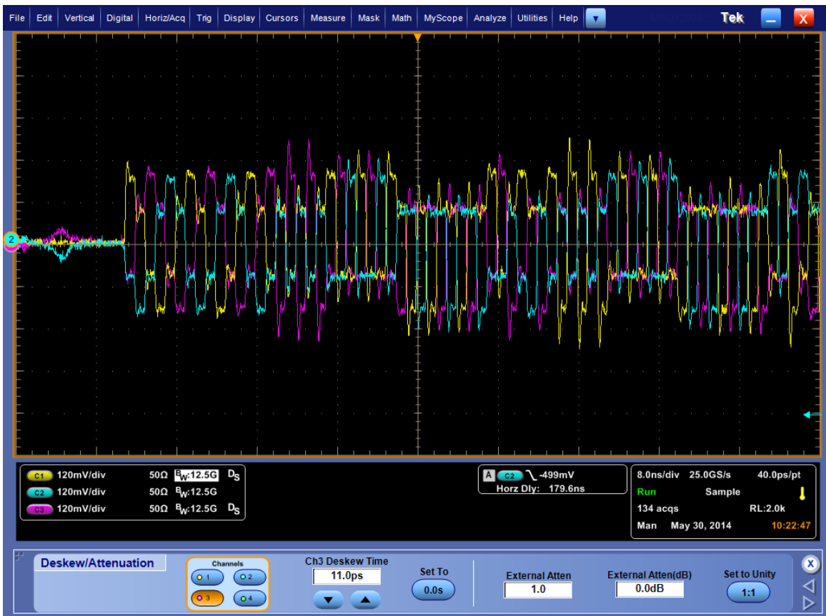
ATx 1.3 Transmitter: Packet through header Yellow: Wire A; Blue: Wire B; Magenta: Wire C Corresponding Received waveform below Yellow: A-B; Blue: B-C; Magenta: C-A
